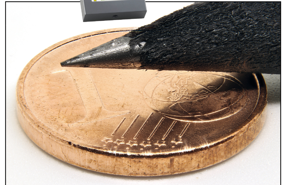
Fig. above: Result of the stack of 100 exposures at f-stop 8, magnification approx. 1: 1, step length 0.1563 mm, camera with APS-C sensor size and 50mm lens in retro-position (NOVOFLEX reverse adapter EOS-RETRO).
